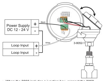
• When the 2350 includes a junction box, connect the 2350 terminals to a loop device as shown.
