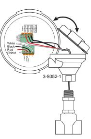
• When the 2350 includes a junction box, connect the 2350 terminals to any Digital (S<sup>3</sup>L) I/O port as shown.
